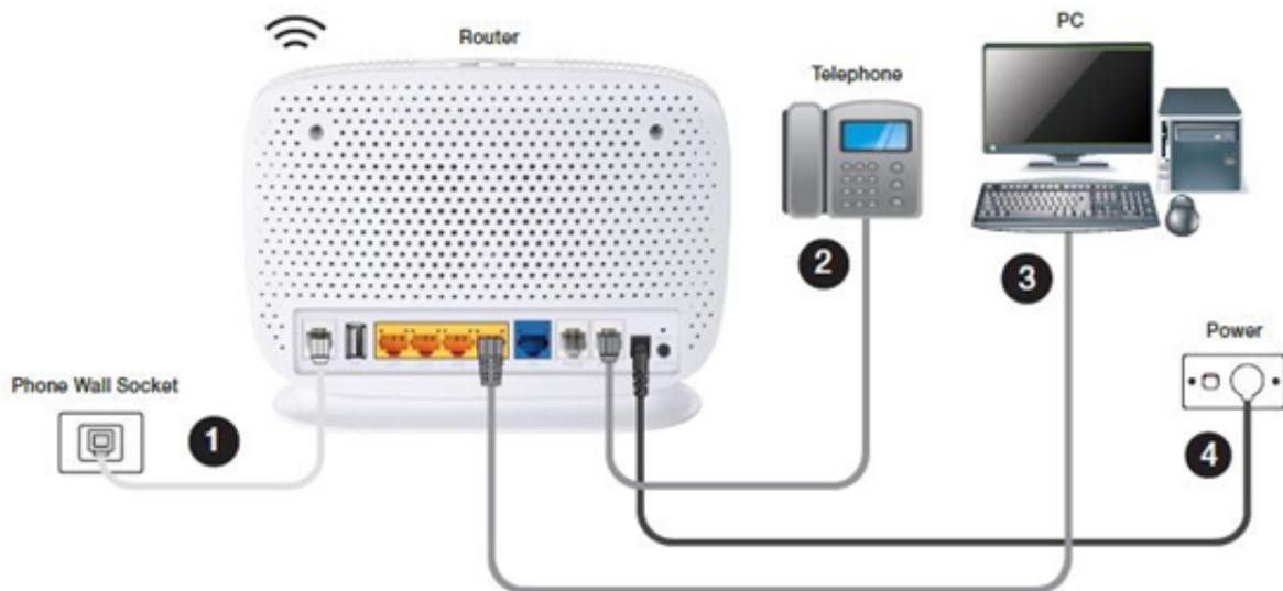
1. Using your gray telephone cord, connect the main telephone socket to the DSL port on the modem.
