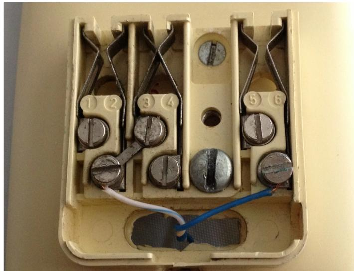
These old sockets were designed for phones with 600-series plugs, which are now largely obsolete. Modern devices use RJ11, RJ12, or RJ45 plugs.
