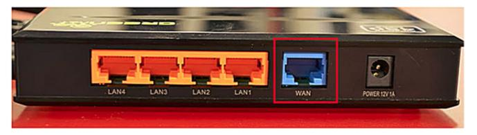
Some modems have both of these ports, and some only have one. To identify which port is required for your nbn type of service, check the table below.
