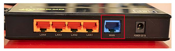
Some modems have both of these ports, and some only have one. To identify which port is required for
