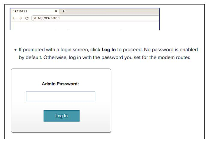
If the IP address does not work, please check the label attached to the back of the modem/router. Else, check your router's IP address. For instructions, click<u>here</u>.
