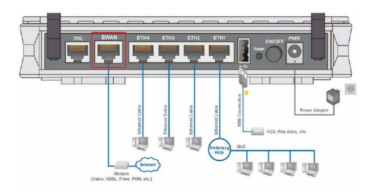
Some modems have both of these ports, and some only have one. To identify which port is required for your nbn type of service, check the table below.
