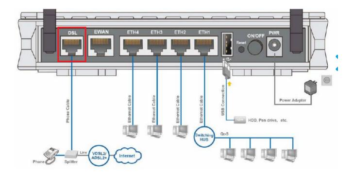
**2.** WAN port - Also known as the internet port that uses RJ-45 Ethernet cable to connect your Billion modem to the nbn connection device.
