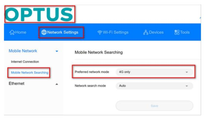
Make sure that the **Preferred Mode** under **Network** is set to **4G** with **2300** (if address shows high indoor, no NQR/Outage for 2300 Mhz) or **4G Only** (if address shows high indoor, no NQR/Outage 1800 Mhz/700 Mhz) and click **Apply** and **OK.**
