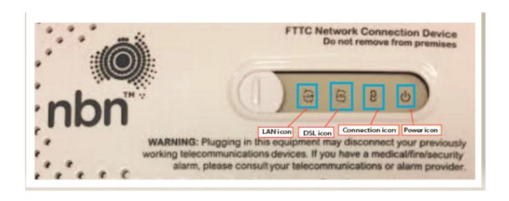
3. The same should be done to the **DSL** light. If the light is **Blue**, it means that there is a connection to the nbn network. If it is **Off**, check for any issues on the telephone cable. If it is still the same, contact us to lodge a fault.
