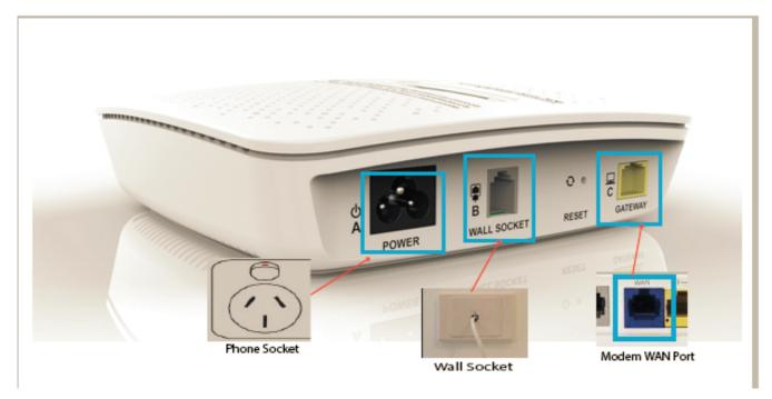
2. Check **Connection** light. If the light is **Blue**, it means that there is a connection to the nbn device on the pit. If it is **Red** or **Off**, try checking the telephone line if it is properly inserted to the wall socket and on the nbn box. If it is still the same, contact us to lodge a fault.
