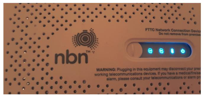
4. Lastly, check the LAN light. A Blue or Amber indicator means that your router has been detected successfully by the nbn box. Otherwise, you might want to check for possible issues with the Ethernet cable.
