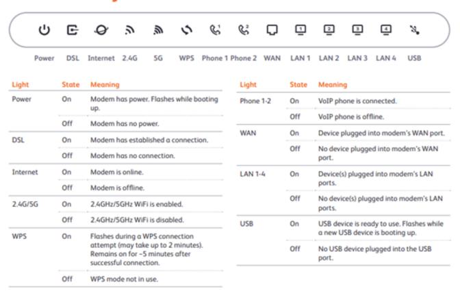
1. Check if the **DSL** light is solid Green. If it is Flashing or Off, check the telephone cable for any issues. You might want to check for other telephone wall socket on your premise.
