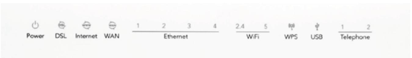
1. Make sure that the modem is turned on. The power indicator should be colored Green. If it is Red/Off, it might have issues with the power connection. Check the power cable if it is properly connected to the power
