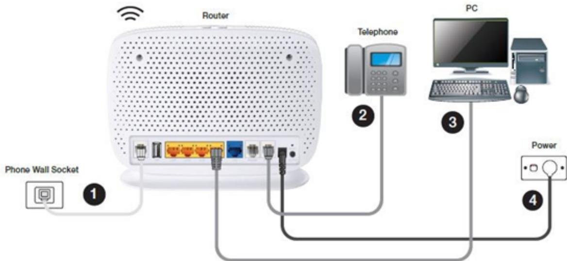
3. If you are using a phone service, connect your phone to the green "Phone" port on the modem using a phone cable.
