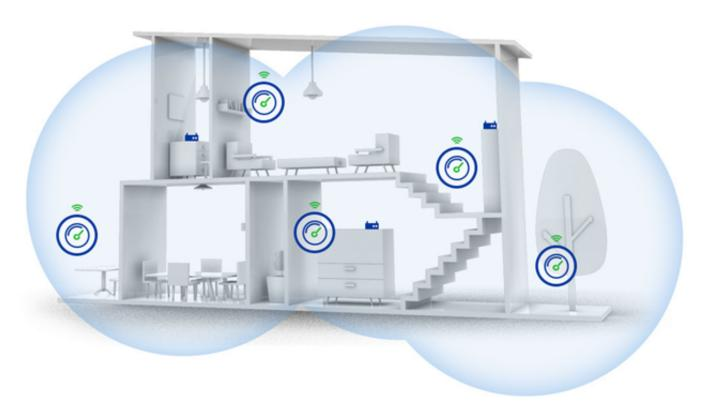
A **mesh network** is a network in which devices -- or nodes -- are linked together, branching off other devices or nodes. These networks are set up to efficiently route data between devices and clients. A mesh network will contain a group of devices that act as a single Wi-Fi network. This provides multiple sources of Wi-Fi around your house, instead of just a single router.
