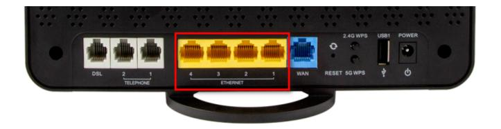
2. Connect the other end of the Ethernet cable to an Ethernet port on your computer or laptop
