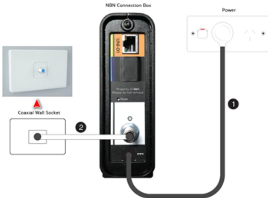
2. Connect the power cable to the black port on the **nbn™** box and the other end to the power outlet.
