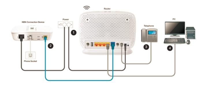
1. Connect your **nbn**<sup>TM</sup> connection box to the main telephone socket using a gray telephone cable.
