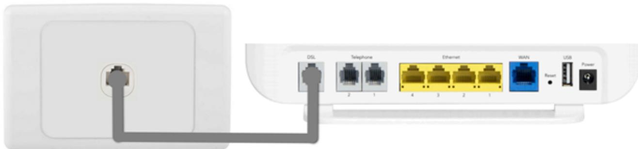
If there is an **nbn** Connection Box installed, you'll need to **connect an ethernet cable from the WAN port on the back of your modem** to the port on the **nbn** Connection Box. This is applicable for FTTP (Fibre to the Premises), Fixed Wireless, HFC (Hybrid Fibre Coaxial), and FTTC (Fibre to the Curb) **nbn** connection types.
