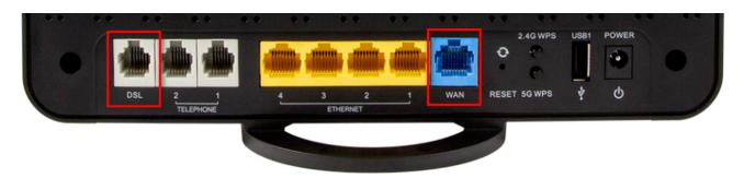
Some modems have both of these ports, and some only have one. Check out the table below to see which port your modem will need to have to connect to
